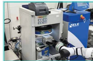
Automated Concrete Cube Testing System
