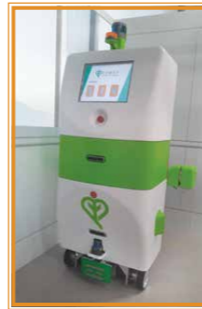
Smart Robotics Coordination System (SRoCoS) for Hospital Logistics 應用於醫院物流的智能機械人協調系統
