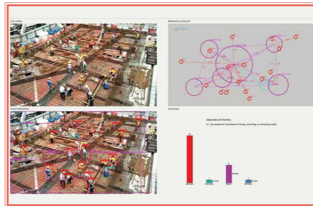
A computer vision-enabled digital twin for construction resource and progress management 施工資源與進度管理數字孿生技術研究
