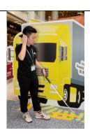
The "Smart Blind Cane" provides voice instructions to the visually impaired when the guiding stick sensed the RFID tags of the tactile paving.
